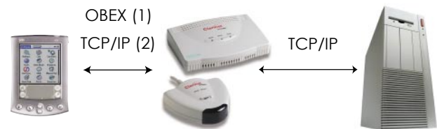
(1) Information Exchange and Network Access By OBEX and TCP/IP (2) Network Access By TCP/IP/PPP
